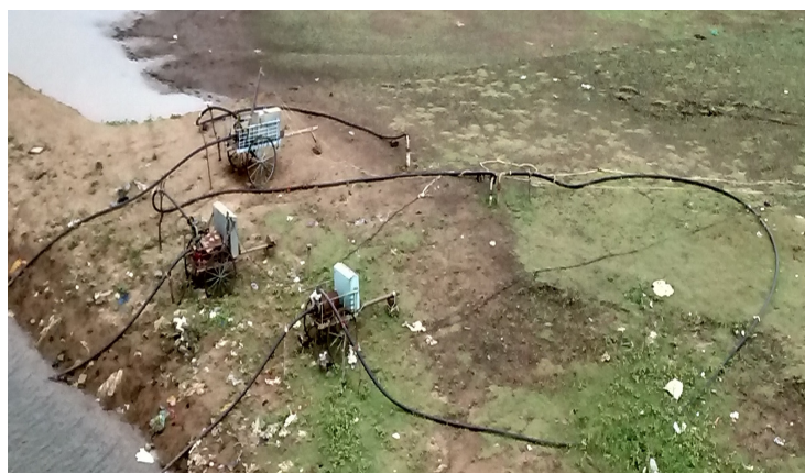
Photo showing an unauthorised IP connection (including motors and portable transformers) – dated April 2015
